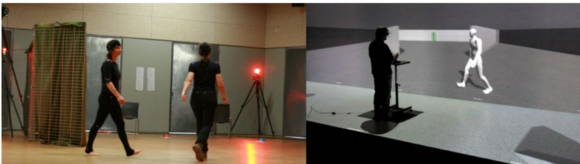
Fig. 1. Left: real experimental situation where two individuals walking at a 90° angle have to avoid each other. Right: virtual experimental situation where a real participant has to avoid a virtual pedestrian in VR application [OBKP17].
